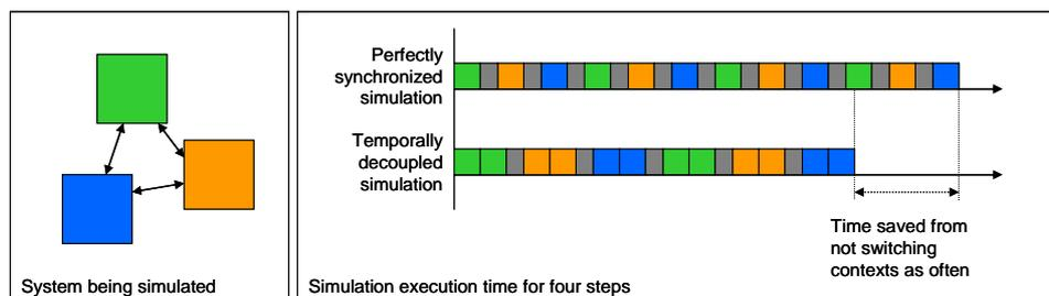
The simple illustration above shows the idea. Here, each part of the simulation runs two steps instead of a single step each time it is invoked. The reduced number of context switches makes the simulation run significantly faster, even without accounting for the efficiencies of enhanced locality. The length of time a simulation part is allowed to run ahead from the other parts is usually known as the **quantum**.
