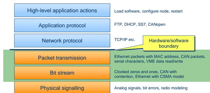
The most detailed modeling level is the **physical signal** level. Here, the analog properties of the transmission medium and how signals pass through it is modeled. This makes it possible to simulate radio propagation, echoes, and signal degradation, or the electronic interference caused by signals on a CAN bus. It is quite rarely used in the setting of developing embedded systems software, since it is complex and provides more details than strictly needed.
